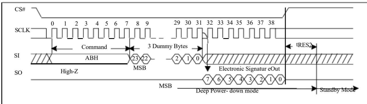
**Figure 5-24b Release from Deep Power-down (RDP) Sequence (Command AB)**
