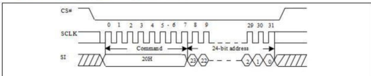
The self-timed Sector Erase Cycle time ( $t_{SE}$ ) is initiated as soon as Chip Select (CS#) goes high. The Write in progress (WIP) bit still can be checked out during the Sector Erase cycle is in progress. The WIP sets 1 during the  $t_{SE}$  timing, and sets 0 when Sector Erase Cycle is completed, and the Write Enable Latch (WEL) bit is reset. If the sector is protected by BP4, BP3, BP2, BP1, BP0 bits, the Sector Erase (SE) instruction will not be executed on the sector.
