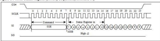
Figure 5-7 Write Status Register (WRSR) Sequence (Command 01)
