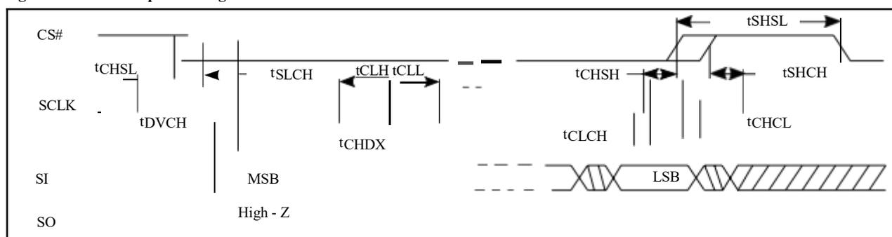
Figure 4-5 Output Timing
