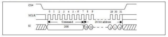
The self-timed Sector Erase Cycle time (tSE) is initiated as soon as Chip Select (CS#) goes high. The Write in progress (WIP) bit still can be check out during the Sector Erase cycle is in progress. The WIP sets 1 during the tSE timing, and sets 0 when Sector Erase Cycle is completed, and the Write Enable Latch (WEL) bit is reset. If the sector is protected by BP4, BP3, BP2, BP1, BP0 bits, the Sector Erase (SE) instruction will not be executed on the sector.
