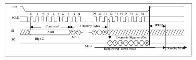
Figure 5-24b Release from Deep Power-down (RDP) Sequence (Command AB)
