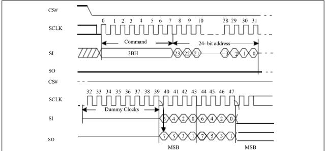
Figure 5-10 Dual Read Mode Sequence (Command 3B)
