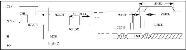
Figure 4-5 Output Timing
