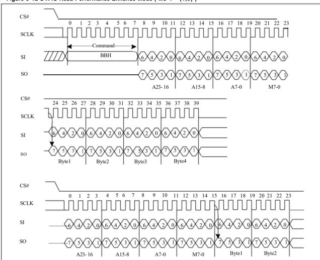
Figure 5-12 2 X IO Read Performance Enhance Mode ( M5-4 = (1,0) )
