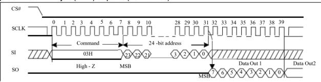
Figure 5-8 Read Data Bytes (READ) Sequence (Command 03)
