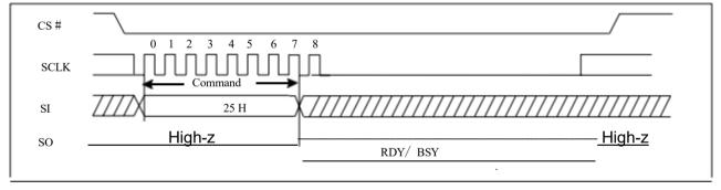
Figure 5-6 Active Status Interrupt (ASI) Sequence (Command 25)
